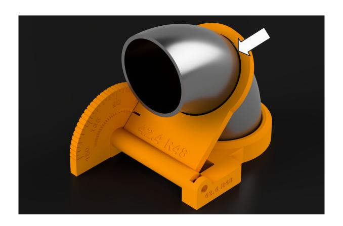
3. Insert the pipe bend and mark along the line. Done!
